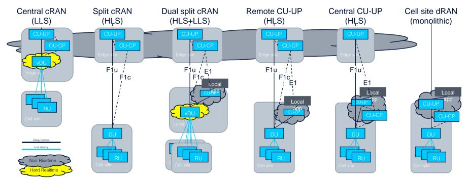
DU: Digital Unit, CU: Central Unit, RU: Radio Unit. UP user plane, CP control Plane
