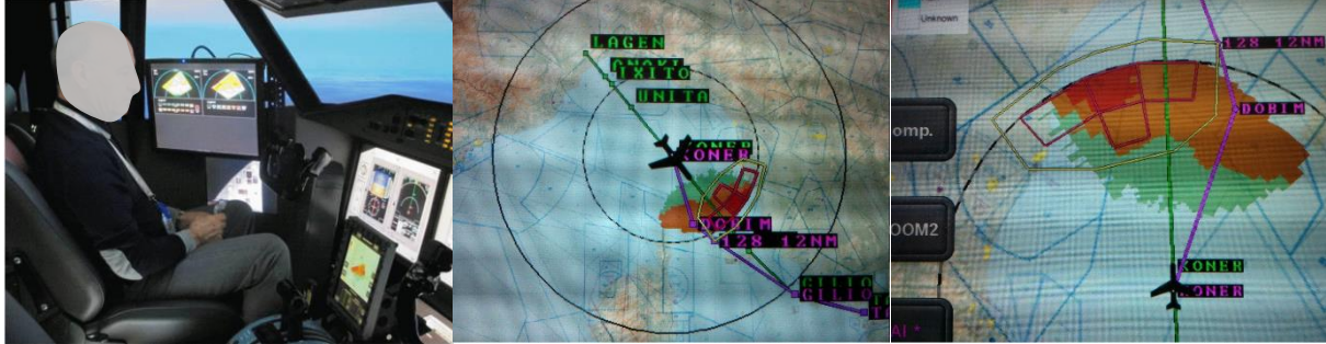
Figure 1: Position of EFB on the cockpit (left) (from [2]) and display of the classification results with identification of risk zones and route suggested to pilot. Two different display and zoom options can be used (center and right panels)
