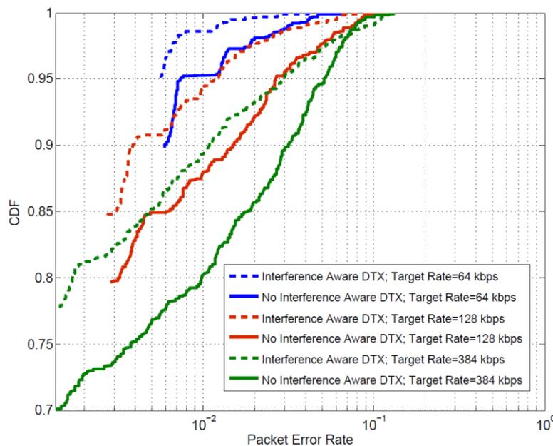
Figure 5. CDF of the Packet Error Rate for different QoS target rate with and without interference awareness mechanism.
