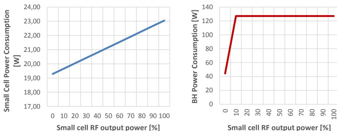
Figure 1. Small-cell and associated microwave BH power consumption [5].
