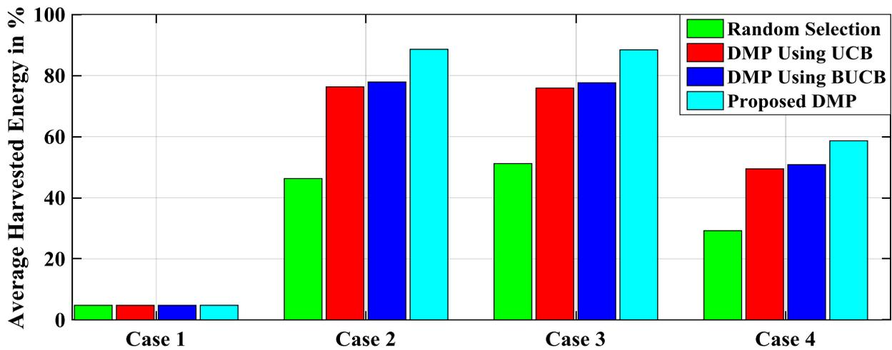
Fig. 2. Average harvested RF power using different DMPs in % with respect to the power harvested using Genie-aided DMP for four different cases of distributions,  $\mu$ .
