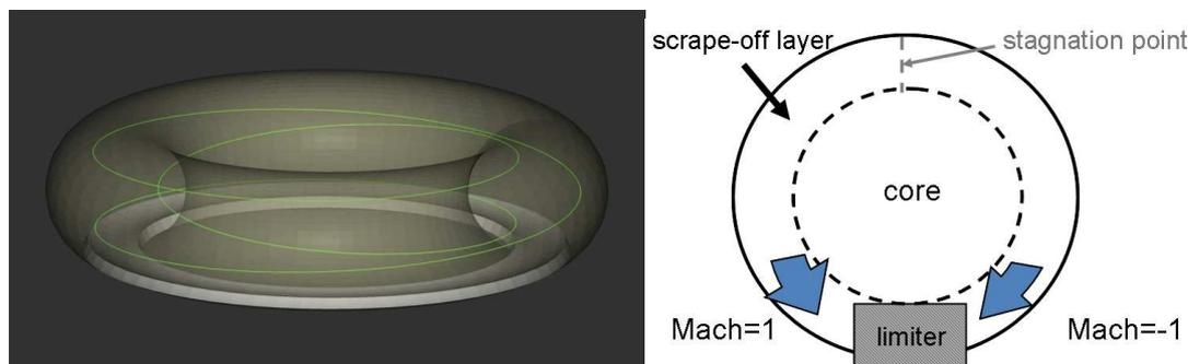
FIG. 1 – Left panel: three-dimensional representation of the tokamak vacuum chamber, with the limiter lying at the bottom of the torus. A magnetic field line is represented in green colour, winding helically around the torus. Right panel: poloidal cross-section of the tokamak. The scrape-off layer corresponds to the area outside the dashed line that denotes the core/SOL transition. In the SOL, parallel flows (flowing along field lines, and therefore poloidally in the cross-section) are driven to
