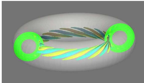
Fig. 2: Decaying mode with toroidal wavenumber 9 in a 3D simulation
