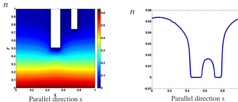
Fig. 3: Left panel: Contour plot of the 2D density field obtained integrating the penalized system given by Eqs. (2) using SOLEDGE-2D code in a geometry with two limiters. Right panel: density profile in the parallel direction for a radial position near the top wall ( $r=0.9$ )
