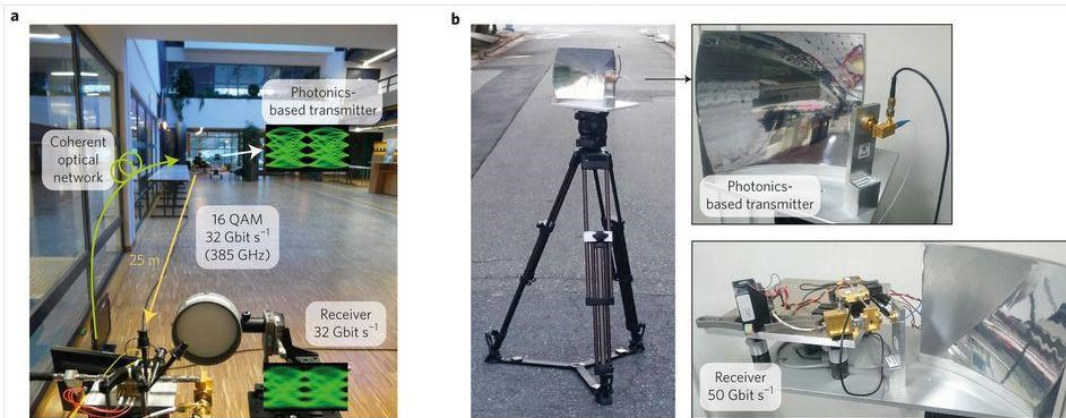
a, Multi-level 32 Gbit s -1 link over 25 m with 16 QAM modulation delivered by a fibre-optic network. b, Real-time 50 Gbit s -1 link over 100 m with OOK modulation.
